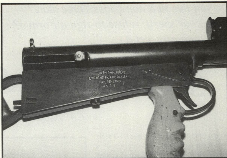
Markings on the trigger frame of the Owen gun at the Champlin Fighter Museum. It reads, "OWEN 9MM MK1.42 LYSAGHT PK. AUSTRALIA PAT. PENDING." The bottom line is the serial number. PK stands for Port Kembla. The Owen gun's tube body, considered the receiver by the B.A.T.F., is unmarked except for the serial number.
