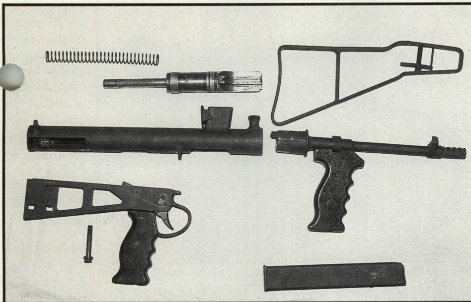
Owen Mk 1 disassembled into its major components.
